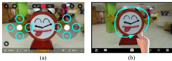
Fig. 2: Compare a common joystick interface and XPose. (a) The left joystick controls the drone’s heading direction and altitude. The right joystick controls its translational movement along or orthogonal to the heading direction. (b) With XPose, the user interacts directly with objects in the photo.
