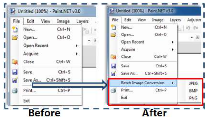
Figure 3: Using WADE, one can easily add an external service to the host program. The utility enabling batch image conversion to JPEG, BMP and PNG is added to Paint.NET by linking to the ImageMagick graphic library.
