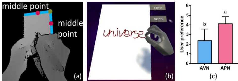
Fig. 10. (a) The construction of the virtual buttons on the augmented physical notepad (APN). A corner (the green dot) and two edge points (red dots) are detected and mapped into 3D space for notepad plane tracking. (b) A user is taking notes with the augmented virtual notepad (AVN). (c) The result of the user study for the augmented notepads .
