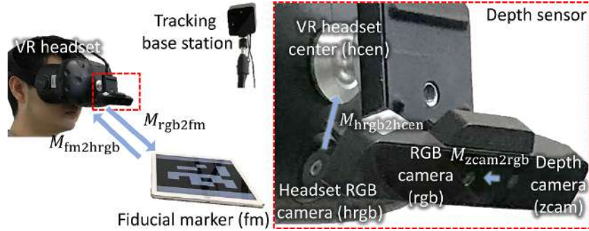
Fig. 2. Our hardware system setup. Note the transformations ( M 's) among various components in the system.
