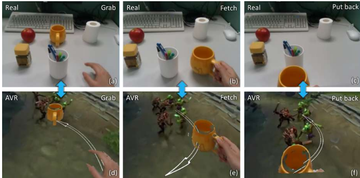
Fig. 6. Illustrating the Target-Hand-Path (THP) incorporation method (the system only incorporates the target object (the cup), the user’s hand and a hollowed guiding path into the virtual environment). The hollowed guiding path helps the AVR user to avoid collision with a physical obstacle located just in front of his/her body during the “grab”, “fetch” and “put back” steps. In addition, only the edges of the guiding path bring in very limited occlusion above the virtual contents.
